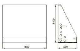
Counterflow device – fitted separately in the counterflow shaft, or in the technology shaft – place the counterflow shafts with the counterflow pipe along the axis of the pool, where the outlets from the counterflow mask are located. This is to achieve the lowest power losses. The maximum distance from the exterior contour of the pool shell is 2000 mm. Should the counterflow be placed away from the axis of the pool shell, its performance will be diminished.
