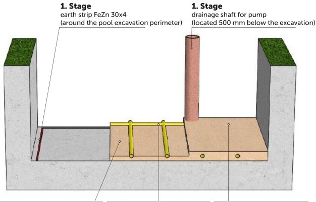
2. Stage gravel backfill (approx. half from a total height of 200 mm)
