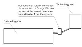
the pipes and discharge of water. For the location of the disconnect fitting, see the picture. The disconnect must be placed at the lowest point of the piping.
