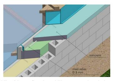
filled – this layer of concrete ensures the stability of the overflow channel. We recommend continuing the concreting only after the concrete layer under the channel has set. During concreting, ensure that the supply cable and the light box are not concreted.
