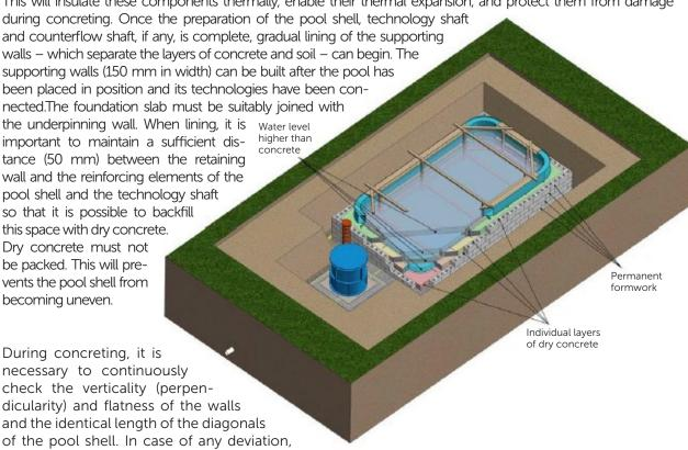
level the shell. Concreting is carried out in layers, keeping the height of a single layer of concrete to a maximum of 300 mm. After each single layer of concrete is completed, the next layer is applied only after the previous layer has set. During concreting, it is necessary to gradually add water to the pool
